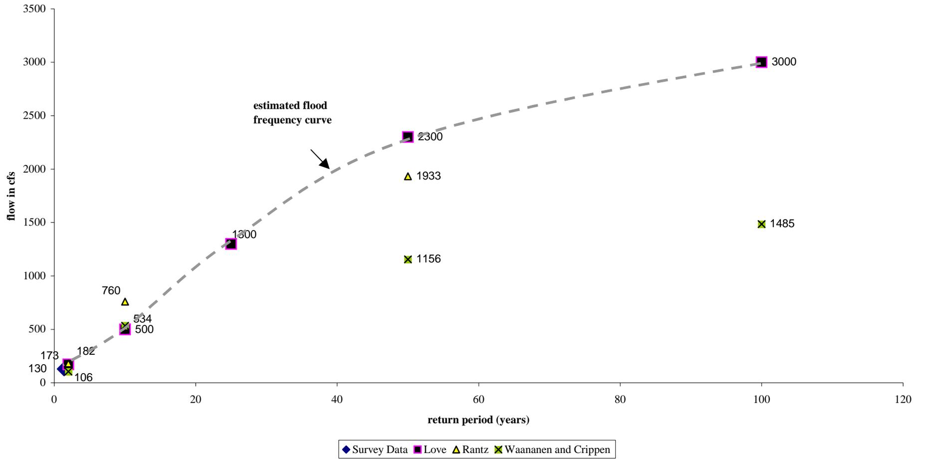
**Figure 8. Estimated Flood Frequency Curve**
